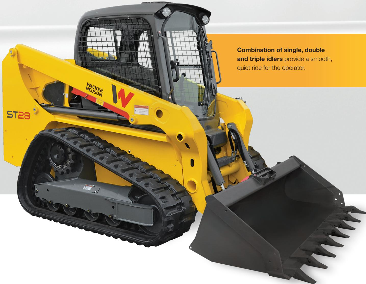
**Combination of single, double and triple idlers** provide a smooth, quiet ride for the operator.
