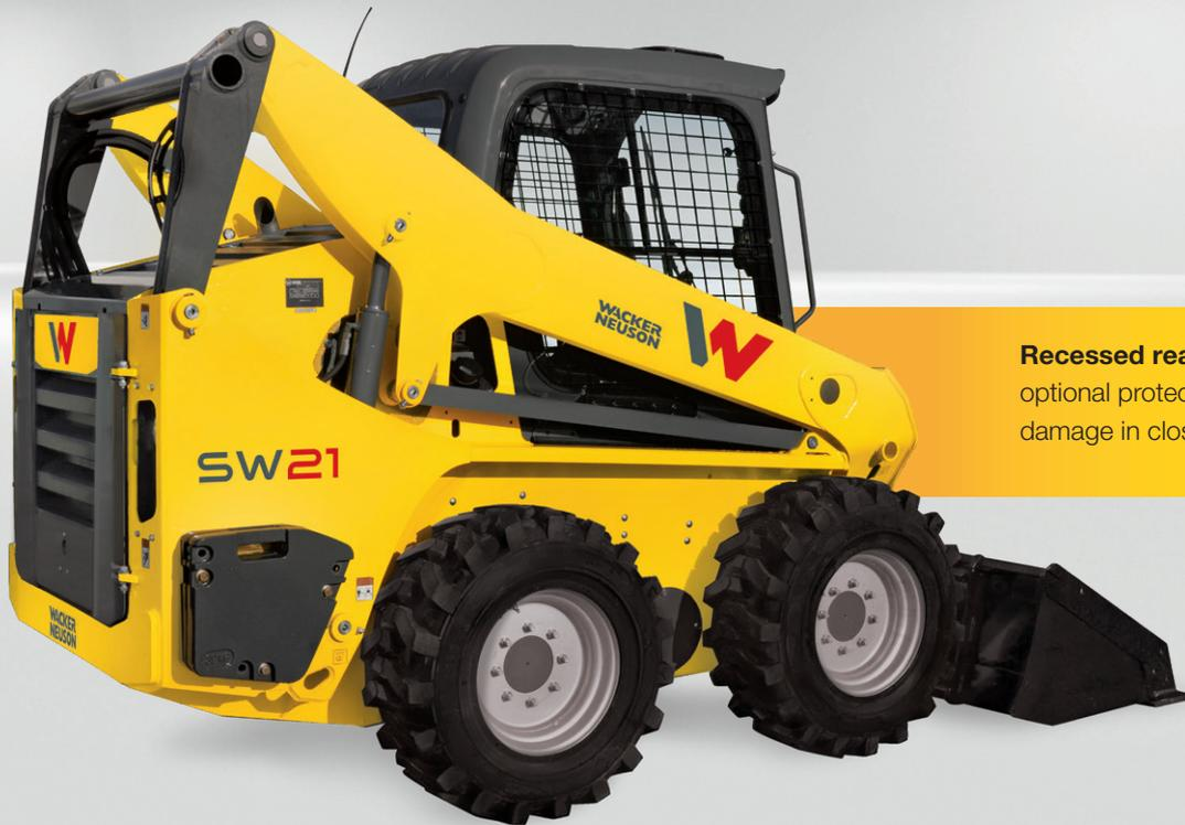
**Recessed rear work lights** with optional protection help prevent damage in close quarters.
