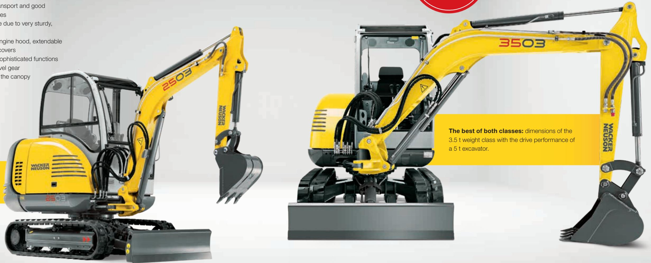
**The best of both classes:** dimensions of the 3.5 t weight class with the drive performance of a 5 t excavator.
