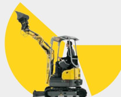
**Complete freedom of movement:** without a tail overhang you can work directly alongside walls.
