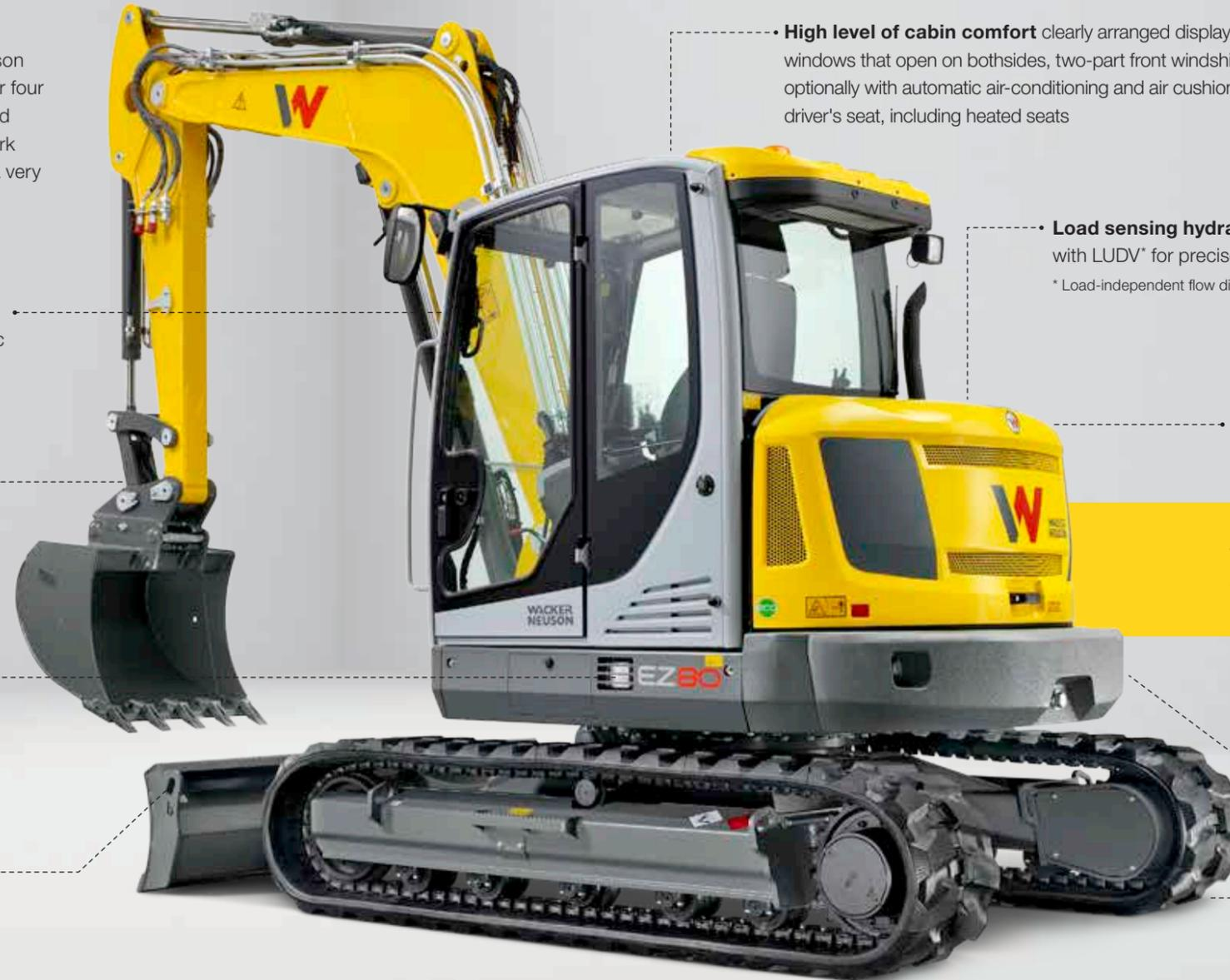
**High level of cabin comfort** clearly arranged display, windows that open on bothsides, two-part front windshield – optionally with automatic air-conditioning and air cushioned driver's seat, including heated seats
