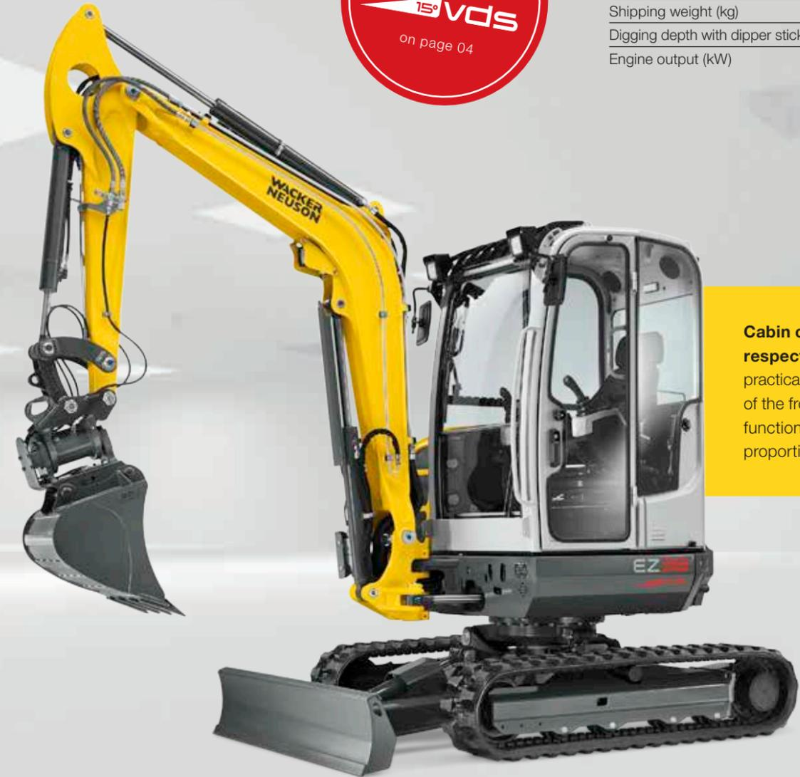
**Cabin comfort in every respect:** enough space, practical splitting mechanism of the front windows and functions such as adjustable proportional control.
