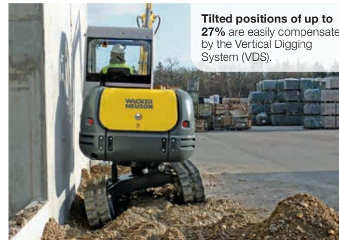
**Tilted positions of up to 27%** are easily compensated by the Vertical Digging System (VDS).
