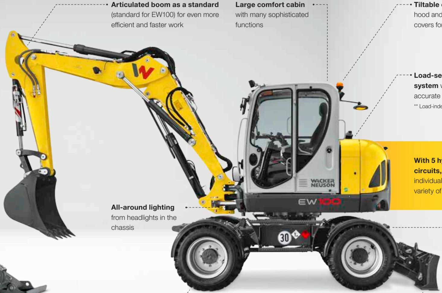
**Articulated boom as a standard** (standard for EW100) for even more efficient and faster work
