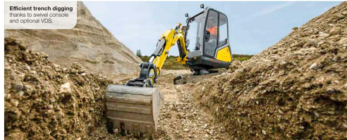
**Zero tail tracked excavator:** optimal when working at the curbside
