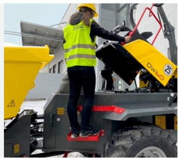
Innovative Dual View concept: 180-degree rotatable operator's seat offers the ideal view when loading and driving
